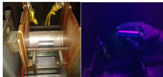
Fig 7 Surface crack test
